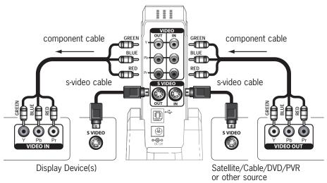
• A signal received at the **Flea** component input in 480i or 576i, will go out from both the component and S-Video outputs. A signal received at the S-Video input in 480i or 576i will go out from both the component and S-Video outputs.
